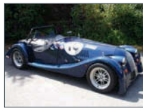
2008. Roadster Lightweight class B race car. Built from a bare chassis by us with great attention to weight saving to full class B spec for the Aero Racing Morgan Challenge Race Series. 4 wheel disc brakes, 7" x 8" Image wheels with Yokohama, modified 3 litre Ford V6, bespoke ECU, race cams, and big bore manifolds circa 2800RPM at 7000RPM. Ready to race.
