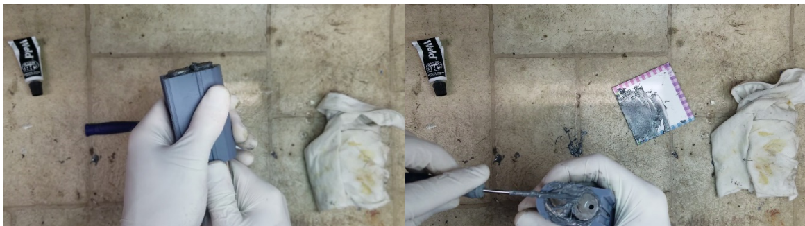
Pulling the bolt rods until they are fully seated.
