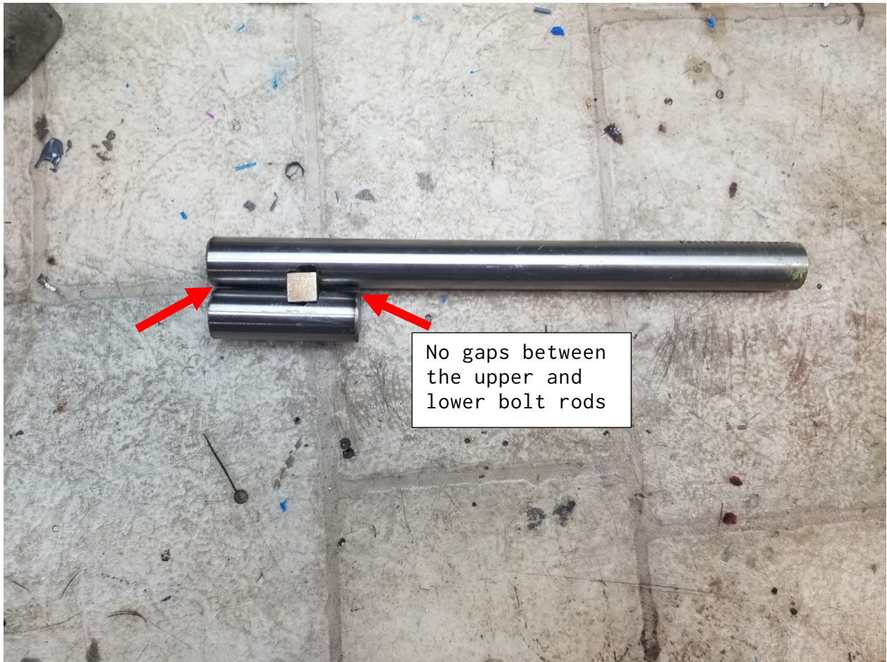
Layout of the weldless bolt. Make sure there is NO gap between the bolt rods. If there is, you need to make the slots deeper.
