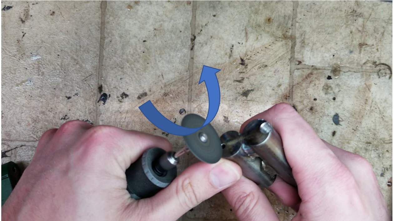
Figure 4: Rounding out the top of the firing pin hole. Use light cuts, starting from the middle of the firing pin hole, and scoop up towards the top of the firing pin hole.
