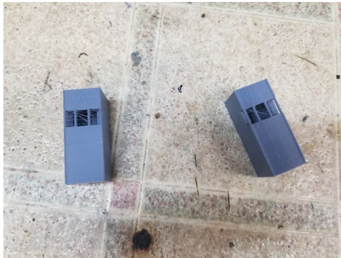
Jigs before removing posts
