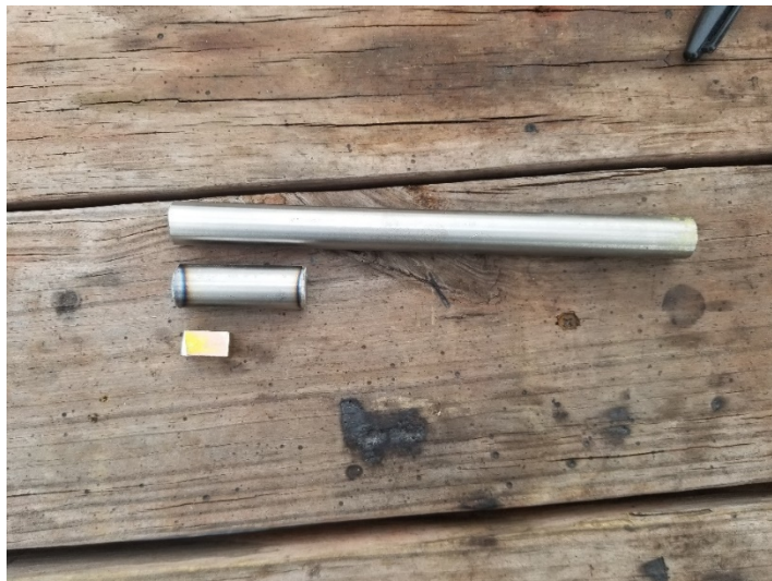
Bolt rods cut to length with bar stock cut to length.
