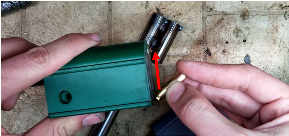
Figure 2: While holding the case at a 45-degree angle to the bolt face, apply moderate pressure (pushing the case against the bolt face) while sliding the case upwards. The case should not snag at any point, but a little resistance or some bumps is fine.
