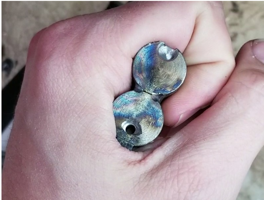
Figure 5: Top of firing pin hole rounded out. Try not to remove more material than this.
