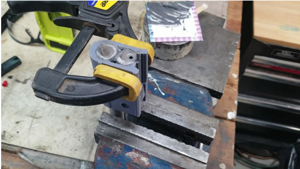
Bolt assembly clamped in place while the JBWeld cures.
