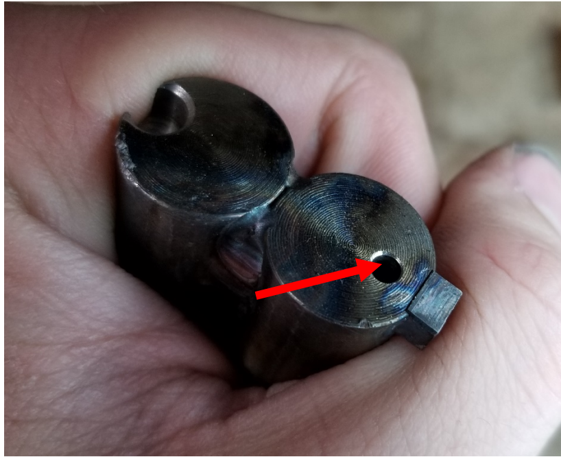
Figure 3: Example of a firing pin hole with a sharp edge. If your firing pin hole has a sharp edge like this and you are having feed issues or feel snagging when sliding cases on the bolt face, you will need to smooth out the top edge of the hole.
