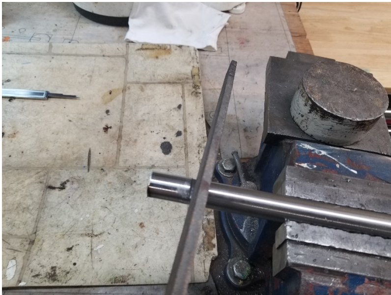
Use a metal file to square up and fine-tune the slot in the bolt rods. File a little, test fit the bar, file some more, etc.
