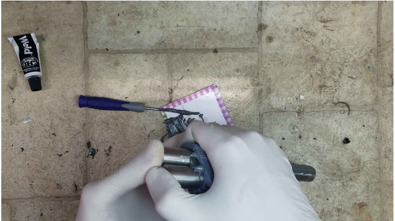
Smush the bolt rods down into the housing. Smear any JBWeld that squishes out onto the bolt rods and back into the housing.
