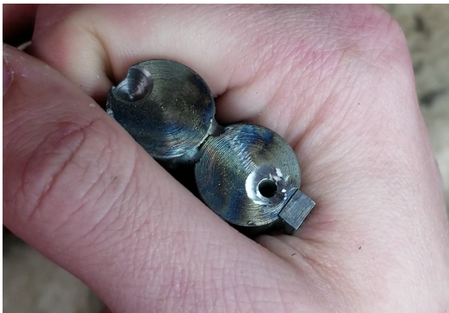
Figure 7: Maximum suggested removal from bolt face.
