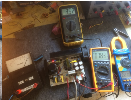
Smps at full peak load, 9.4A Current limit about to cut in at around 10A
