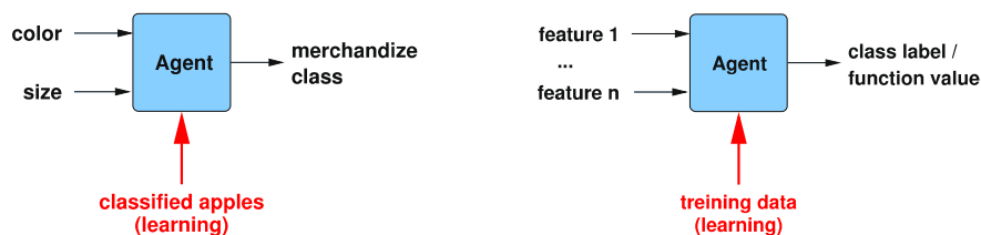
Fig. 8.4 Functional structure of a learning agent for apple sorting ( left ) and in general ( right )
