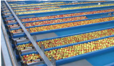
Fig. 8.2 BayWa company apple sorting equipment in Kressbronn and some apples classified into merchandise classes A and B in feature space (Photo: BayWa)
