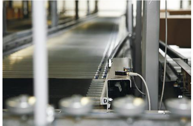
Mini-rectangular plastic, retroreflective photoelectric sensors from AutomationDirect have reliable sensing ranges of 4 m, making them a good fit for detecting the presence of boxes on a conveyor. (Courtesy of AutomationDirect)
