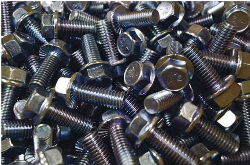
These bolts were barrel-plated with Zn-Ni and trivalent chromate.
