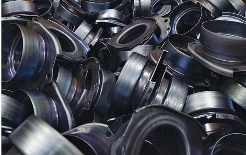
Complex stamped parts were rack-plated with Zn-Ni and trivalent chromate.
