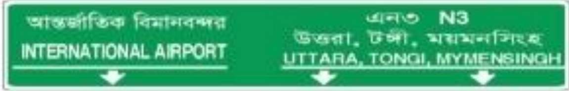
Advance Direction sign Mounted Over head with lane information
