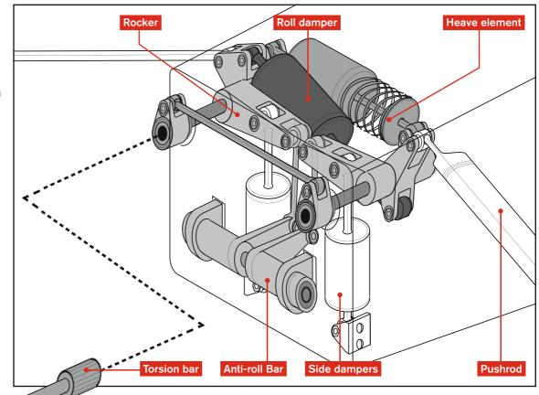
that are twisted by the pushrod/rocker to provide the springing medium. Then, side dampers take car of individual wheel movement.
