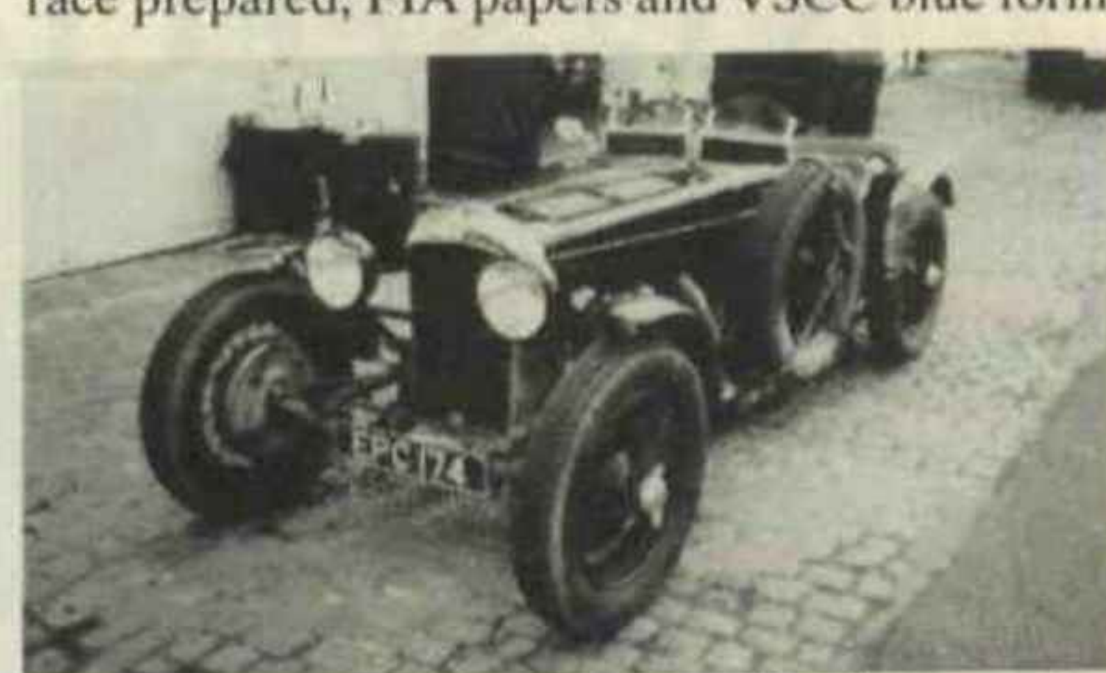
1936 FRAZER NASH. 1500cc Meadows engine with Laystall crankshaft. "Chain Gang" car with TT Replica style body. VSCC and Frazer Nash Section eligible, ex-Paul Emery.
