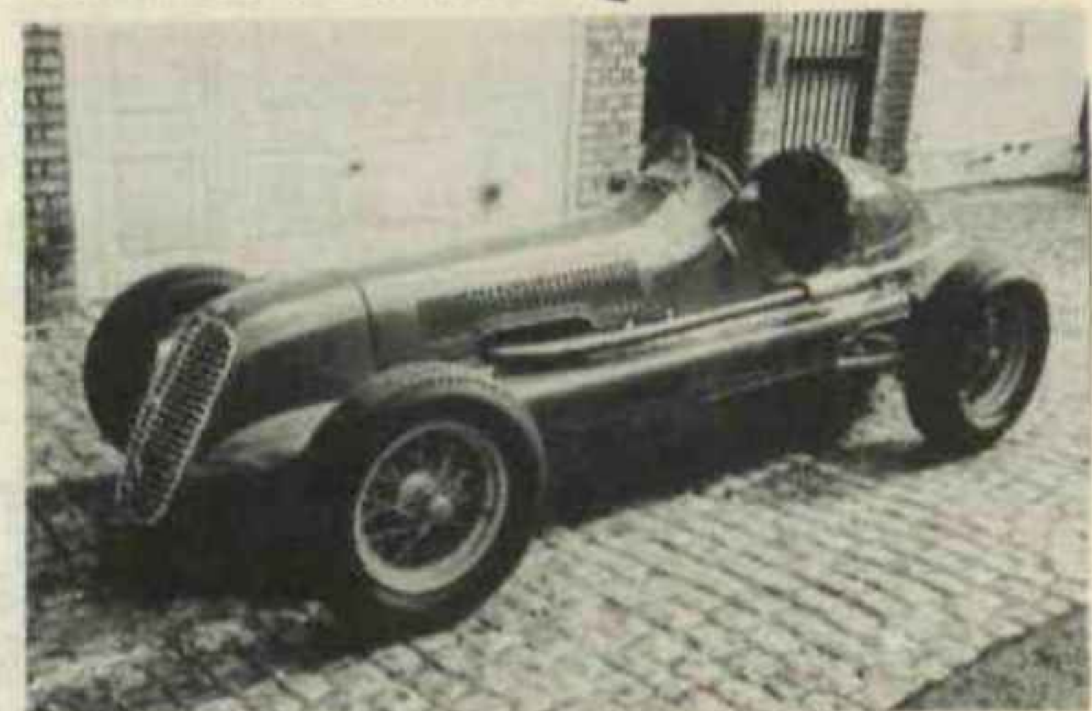
1938 MASERATI 4CM/4CL. 1 1/2 litre, 2 stage supercharged, 16 valve, 4 cylinder Grand Prix car. Chassis and engine to 4CL specification. Fully race prepared, FIA papers and VSCC blue form.
