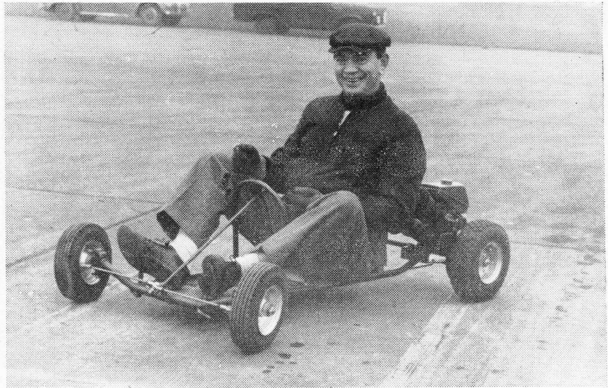
THIS, believe or not, is a "go-cart"—and in tuned form will do 40 m.p.h.! It is powered by a 90 c.c. two-stroke engine, driving one wheel, and has one disc brake. The U.S.A.F. at Burtonwood has five of them and they are raced on a 100 yard bowl. "Driving" this one is Mickey Flynn.
