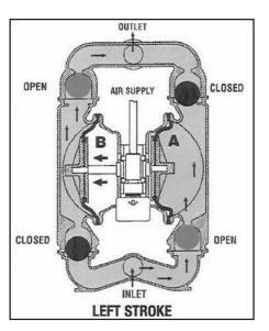
**Figure 3:** At completion of the stroke, the air valve again redirects air to the back side of diaphragm A, which starts diaphragm B on its exhaust stroke. As the pump reaches its original starting point, each diaphragm has gone through one exhaust and one discharge stroke. This constitutes one complete pumping cycle. The pump may take several cycles to completely prime depending on the conditions of the application.
