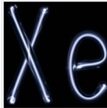
Xenon, operated as a 'neon light,' consists of a collection of mostly spectral lines, missing much of the continuum radiation needed for good color rendering.
