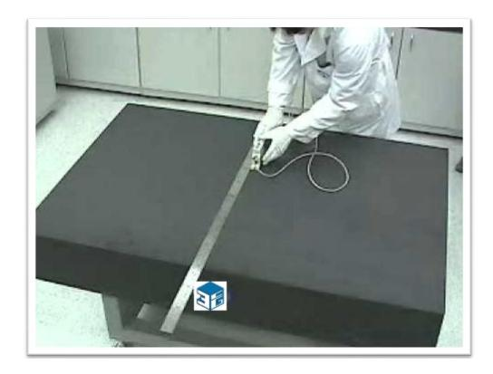
The calibrated yet incredibly flattened veneer of the surface plate provides the inspector with the freedom to use it as a baseline for their procedure of inspection of the instrument calibration.
