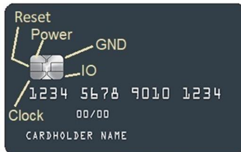
Figure 7 Electrical connections of embedded memory card.
