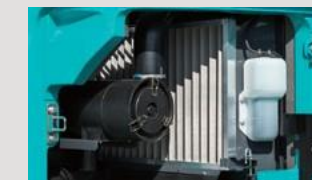
iNDR filter/radiator reservoir tank/air cleaner
