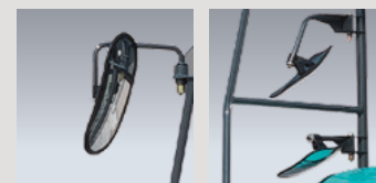
•Rearview mirrors on left and right, and third mirror at lower right optimize visibility and safety.
