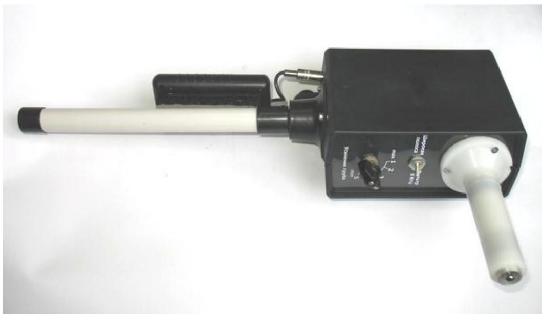
Rice. 118. Meter of electromagnetic geophysical anomalies - VEGA.
