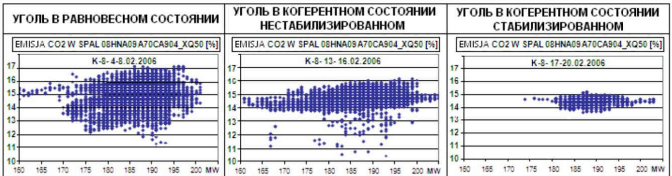
Rice. Fig. 40. Dependence of CO 2 emission on the generated power during coal combustion for equilibrium and coherent states.
