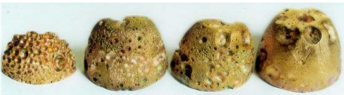
Rice. 51. View of porous copper ingots obtained by processing a copper melt with torsion radiation at various frequencies.
