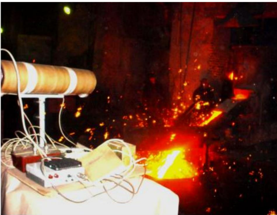
Rice. 55. Treatment of the melt according to the SVM technology of the V.F. Panov group with the generator of S.A. Kurapov. The impact is made through the wall of the metallurgical furnace.
