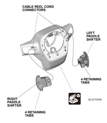
53. Plug-in the new cable reel cord connector.
