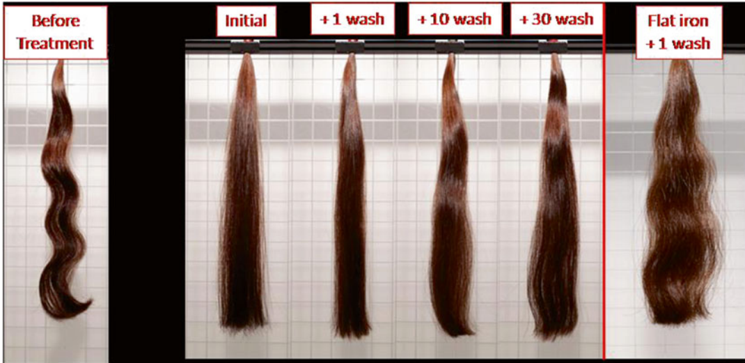
Fig. 3.37 Lab test of Brazilian keratin treatment (BKT), from initial results to noticeable decrease in straightening due to subsequent washings
