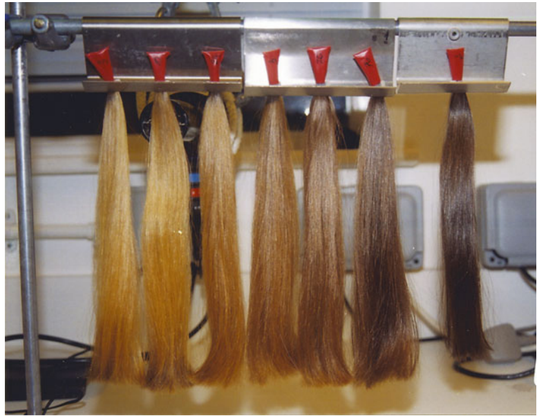
Fig. 4.10 Care is taken to ensure reproducibility of hair source and size of hair tresses. In many cases, hair from multiple women is first screened for low to moderate damage levels and then blended to create a uniform substrate
