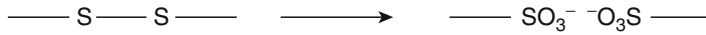
Fig. 3.34 The second chemical effect that the perhydroxyl anion will perform is to break disulphide bonds of the cross-linking amino acid cystine to form cystic acid
