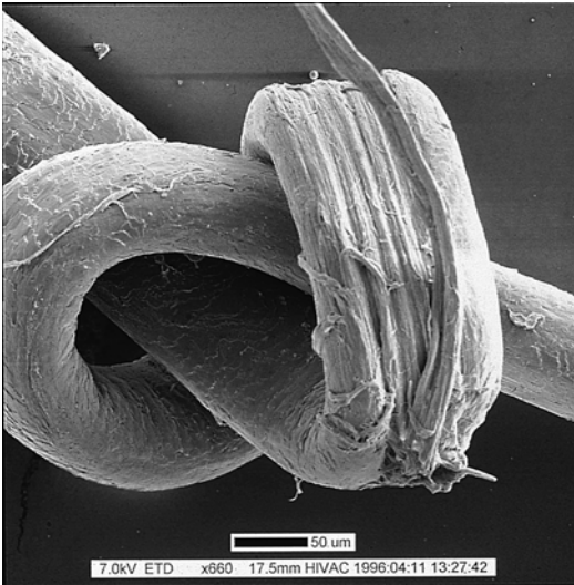
Fig. 3.25 Scanning Electron Microscope image of knots in hair
