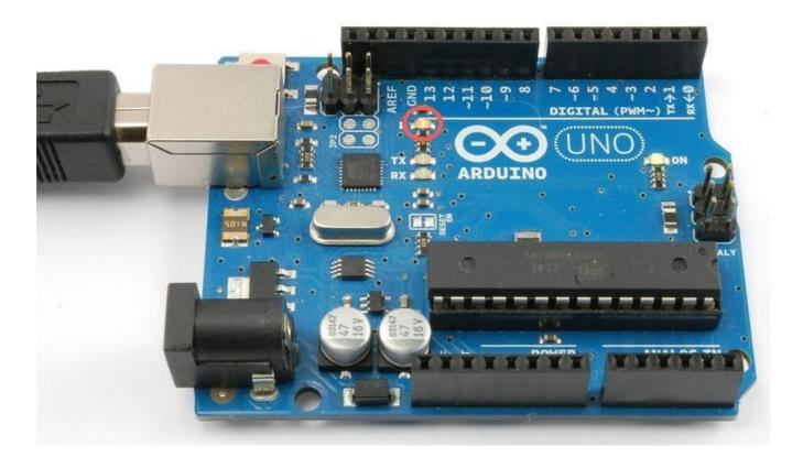
You may find that your Arduino board's 'L' LED already blinks when you connect it to a USB plug. This is because Arduino boards are generally shipped with the 'Blink' sketch preinstalled.
