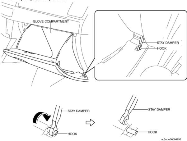
2. Push the glove compartment in the direction of the arrow and remove hooks.
