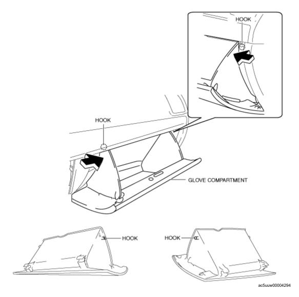
3. Pull down the glove compartment in the direction of the arrow (1).
