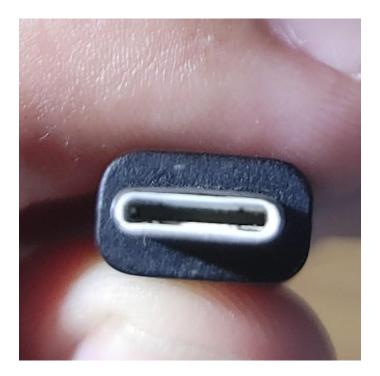
If you pay attention, you can see how the metal part is slightly separated from the plastic part of the connector, this is what we want. All of this is to make sure your USB C connector applies more pressure on your USB C port on your LG v60, so when you charge it, no matter how much you move it around, it won't disconnect.
