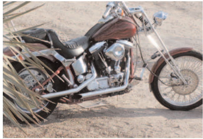
Figure 21.4 Motorcycle fitted with straight mufflers capable of producing noise levels above 100 dB. Photo courtesy J.F. Artiola.
