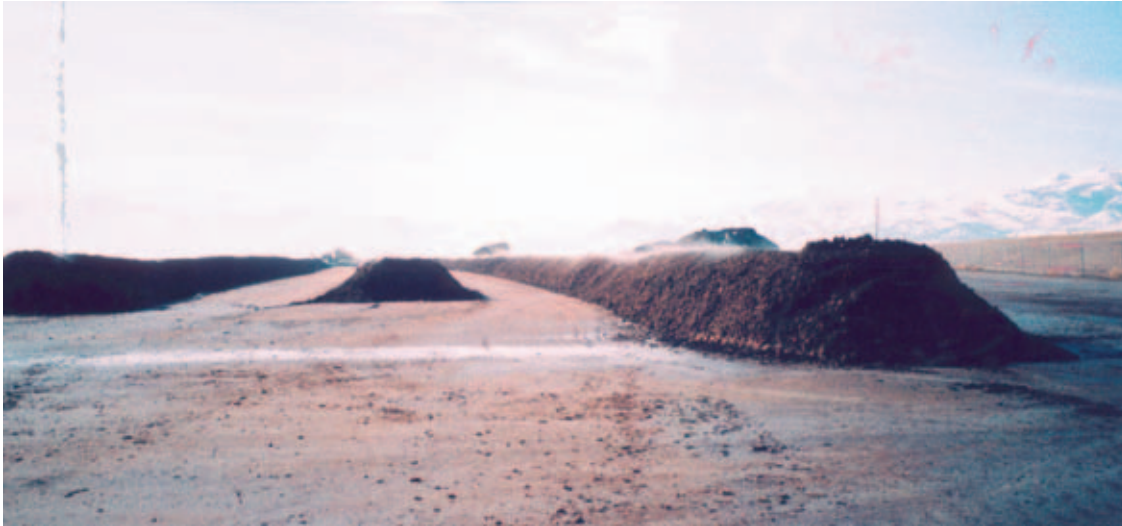
Figure 26.26 Biosolid composting via the windrow process. Here, three windrows are illustrated. Photo courtesy I. L. Pepper
