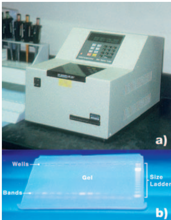
Figure 1.8 (a) An automated PCR thermalcycler that is used to amplify target DNA. (b) A gel stained with ethidium bromide. From Pollution Science © 1996, Academic Press, San Diego, CA.
