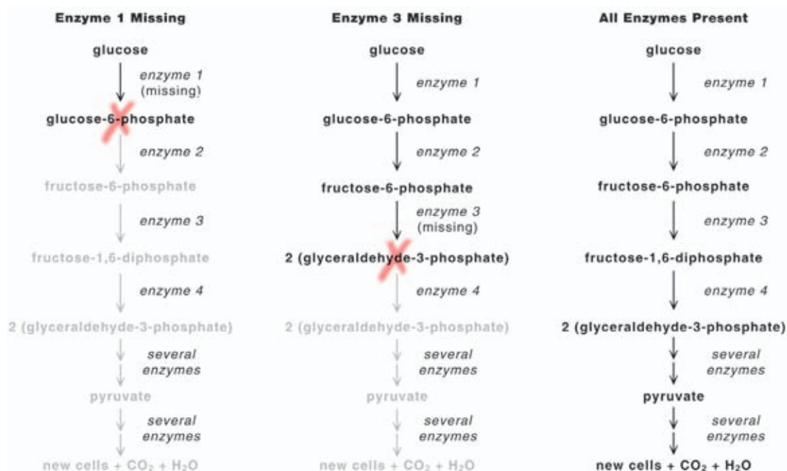
Figure 8.2 Stepwise degradation of organic compounds. A different enzyme catalyzes each step of the biodegradation pathway. If any one enzyme is missing, the product of the reaction it catalyzes is not formed (denoted with a red cross). The reaction stops at that point and no further product is made (shown in gray). From Pollution Science © 1996, Academic Press, San Diego, CA.
