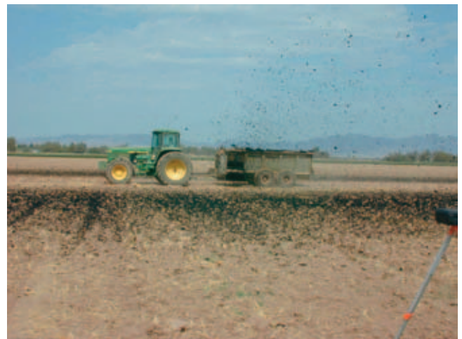
Figure 27.7 Land application of cake biosolids in Eastern Washington. Photo courtesy J.P. Brooks.
