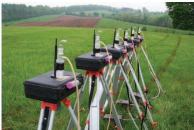
Figure 5.15 Air samplers used to estimate bioaerosol concentrations. From Environmental Microbiology Laboratory Manual, Second Edition © 2004, Academic Pres, San Diego, CA.
