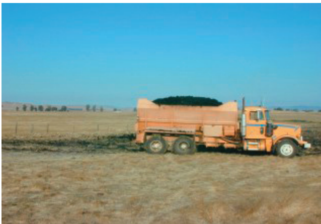
Figure 27.4 Land application of cake biosolids via a manure spreader. Photo courtesy J.P. Brooks.
