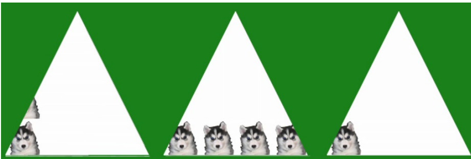
Figure 3-6. Left - TEX_WRAP_S set to CLAMP_TO_EDGE ; Center - TEX_WRAP_T set to CLAMP_TO_EDGE ; Right - both S and T set to CLAMP_TO_EDGE
