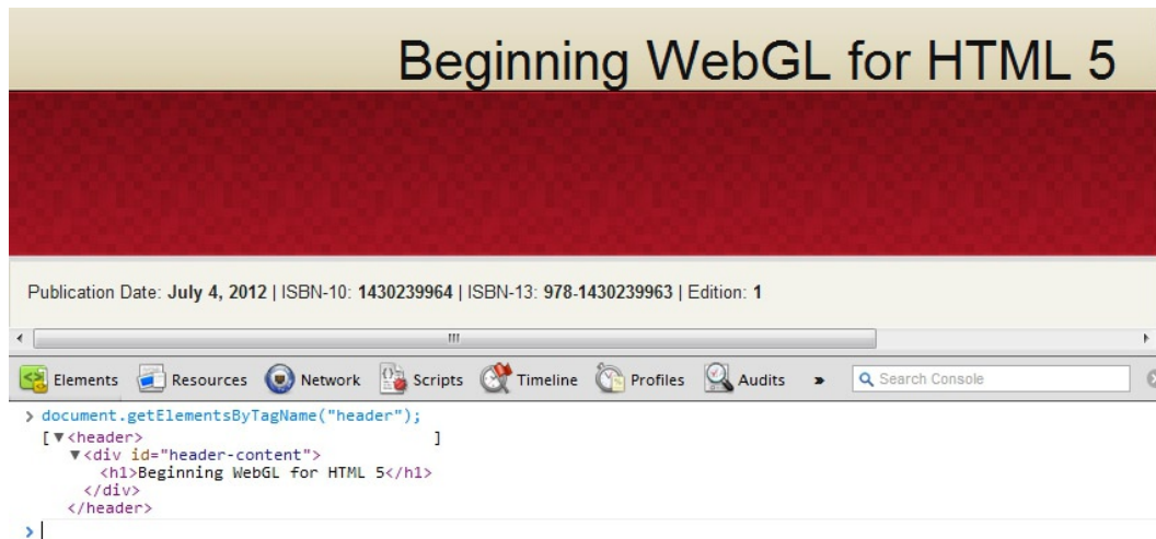
Figure 9-2. Using the console in Chrome Developer Tools to search for the <header> tag
