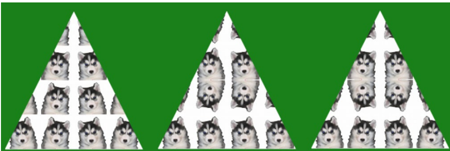
Figure 3-7. Left - TEX_WRAP_S set to MIRRORED_REPEAT ; Center - TEX_WRAP_T set to MIRRORED_REPEAT ; Right - both S and T set to MIRRORED_REPEAT
