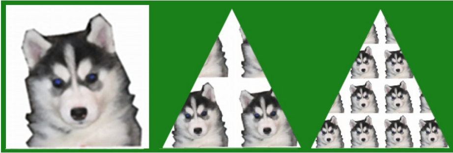
Figure 3-5. Left - original texture image; Center - texture application onto a triangle with default REPEAT; Right - multiplying the texture coordinate values in the shader to pronounce the repetition
