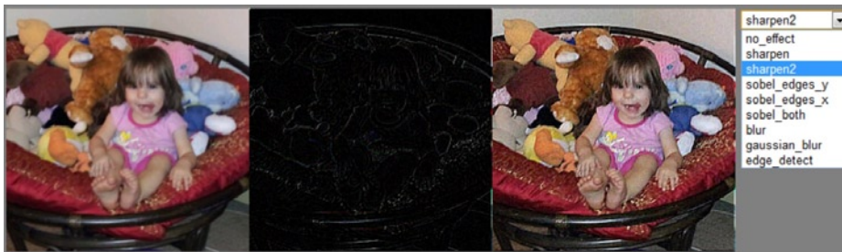
Figure 10-9. A simple GUI that we will build—left: original image; center: kernel matrix effect; right: the effect combined with the original image
