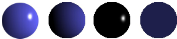
Figure 3-13. Sphere (far left); diffuse reflection (left); specular reflection highlight (right); ambient component (far right)
