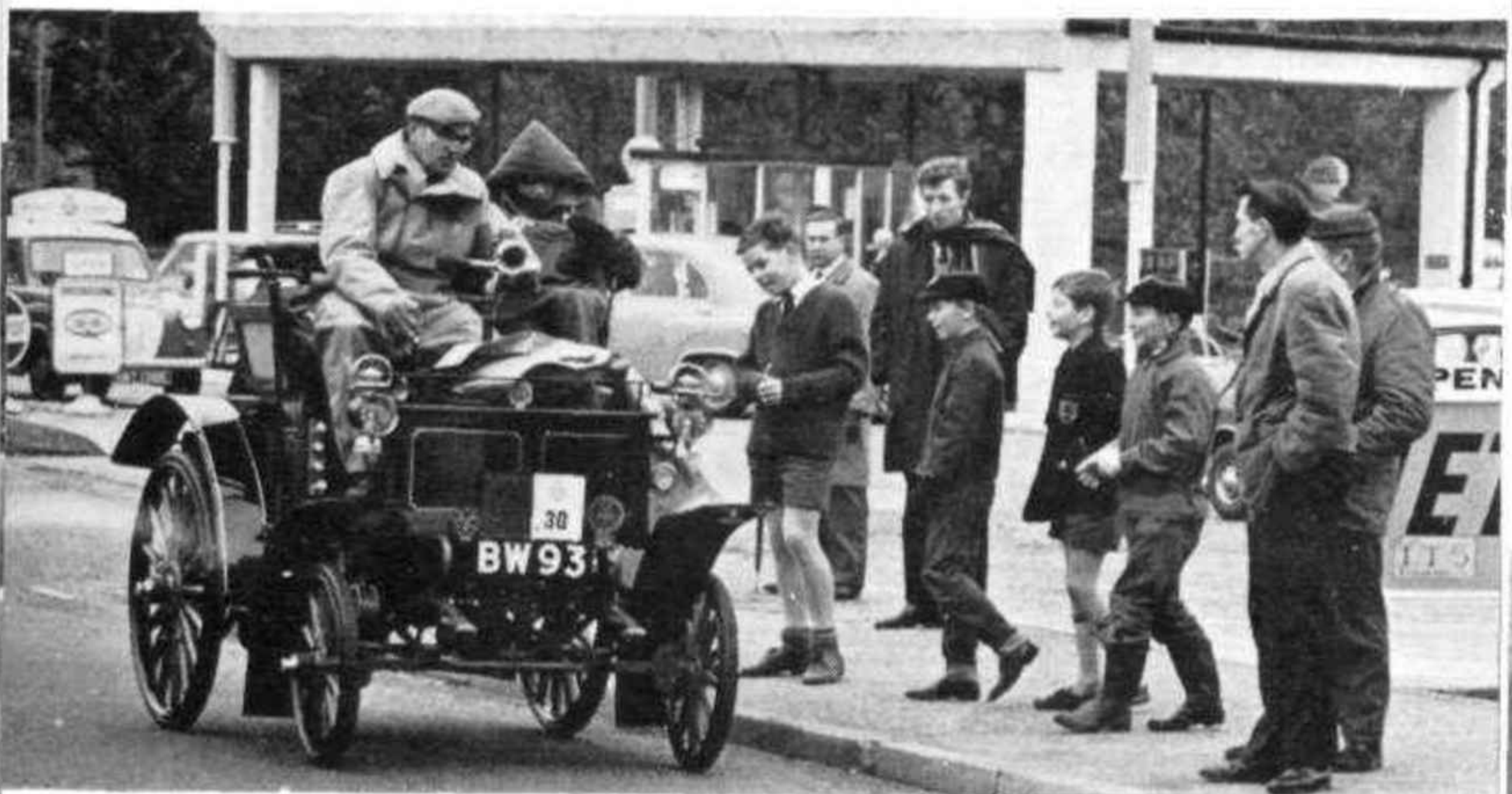
ANCESTOR OF THE REX MOTORCYCLE.—The Northwoods on their 1901 6-h.p. International Charette, which was built in Coventry and known as an Allard. It has belt-drive, from a single-cylinder engine. Note the vertical steering column.
