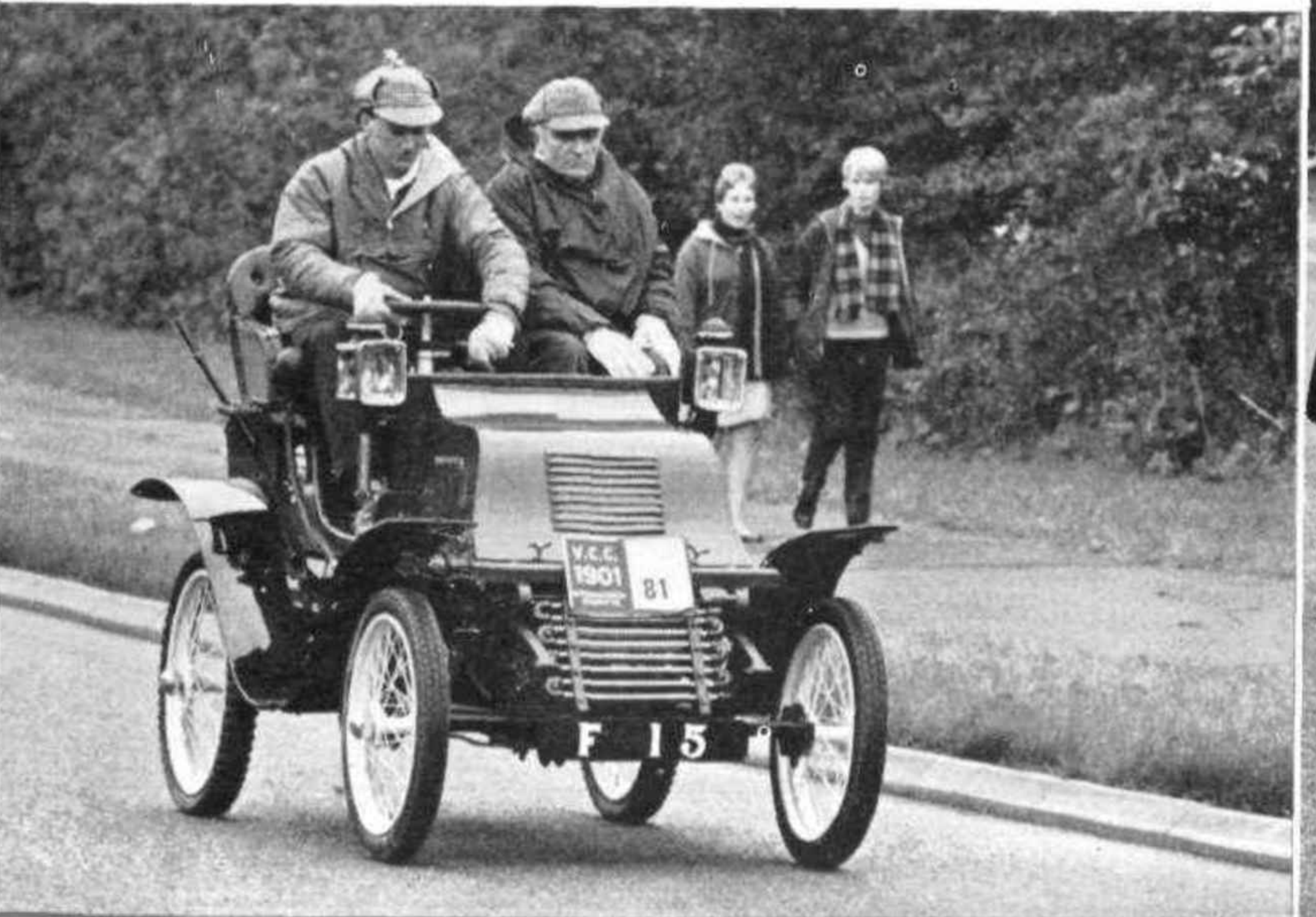
ANCESTOR OF THE REX MOTORCYCLE.—The Northwoods on their 1901 6-h.p. International Charette, which was built in Coventry and known as an Allard. It has belt-drive, from a single-cylinder engine. Note the vertical steering column.
