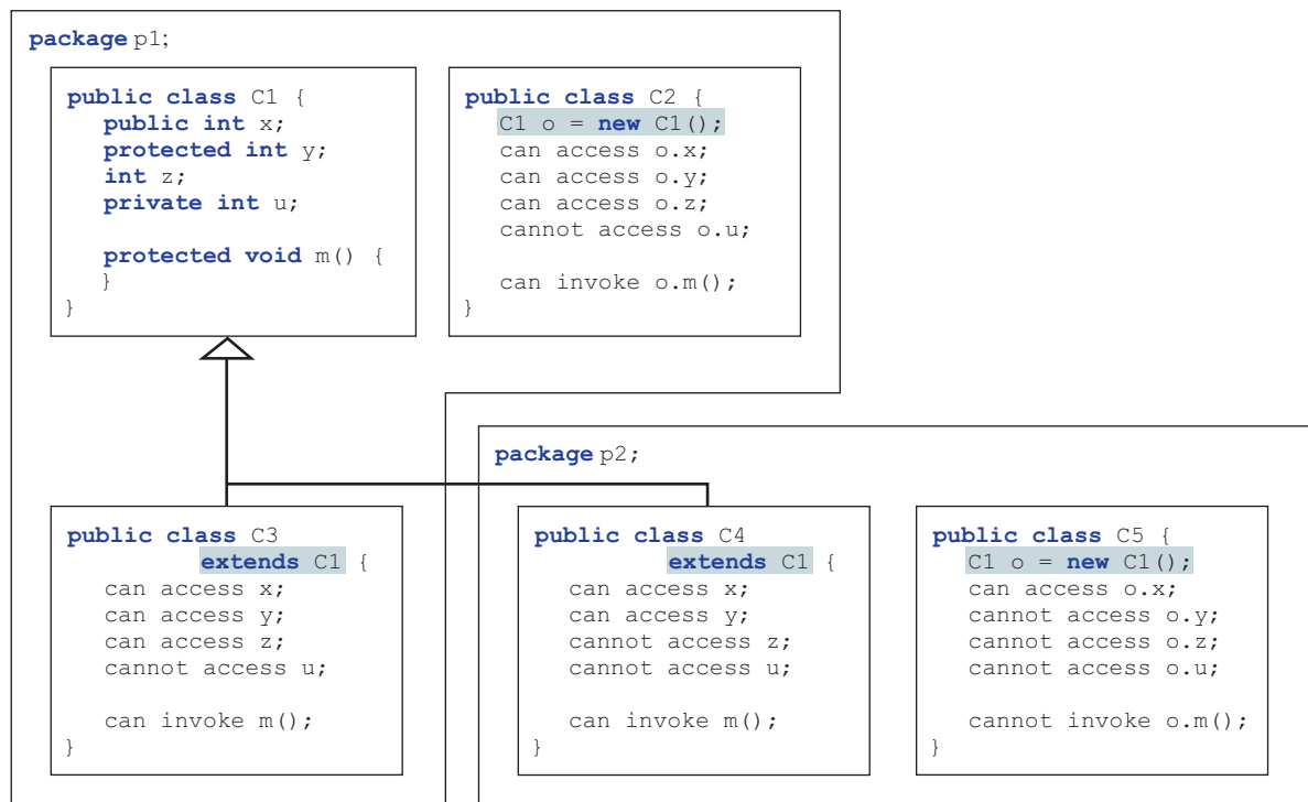
FIGURE 11.5 Visibility modifiers are used to control how data and methods are accessed.
