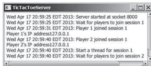
FIGURE 33.15 TicTacToeServer accepts connection requests and creates sessions to serve pairs of players.
