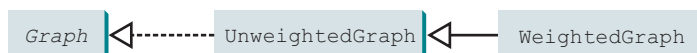
FIGURE 28.8 Common operations of graphs are defined in the interface and concrete classes define concrete graphs.
