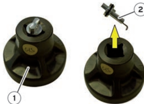
Fig. 170 Wrench for single-bolt wheels, with tool for removing wheel cover/ releasing lock pin.
