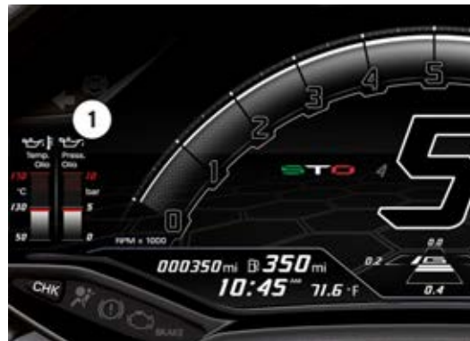
Fig. 14 Instrument cluster: engine oil pressure gauge.
