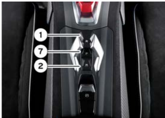
Fig. 106 Reverse gear R selector lever (1), manual gear changing mode M button (2) and parking mode P (7) button.
