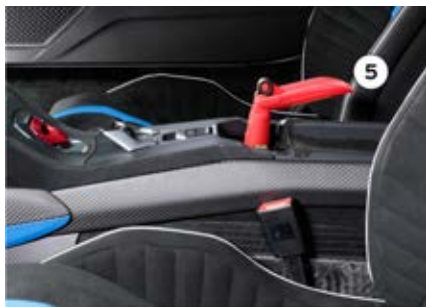
Fig. 188 Disengaging the transmission.
