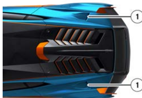
Fig. 150 Air intake ducts (1).
