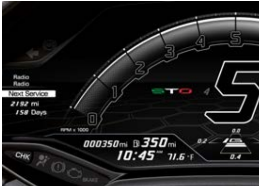
Fig. 33 Instrument cluster: sample display of a maintenance interval.
