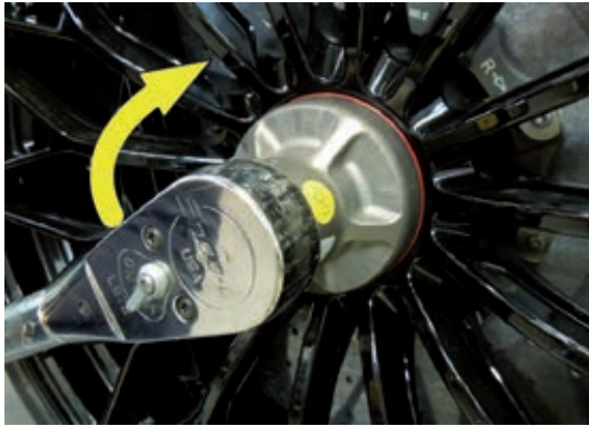
Fig. 175 Tightening the single bolt.
