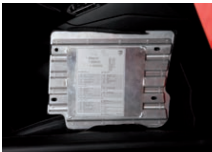
Fig. 191 Removing the fuse access panel.
