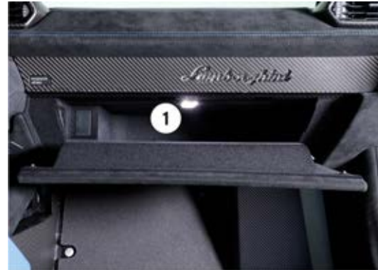
Fig. 67 Glove box on the passenger side: interior light.
