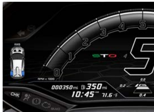
Fig. 32 Instrument cluster: animation of rear wheel steering system.
