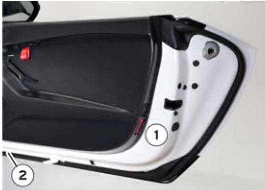
Fig. 66 Door: clearance light.
