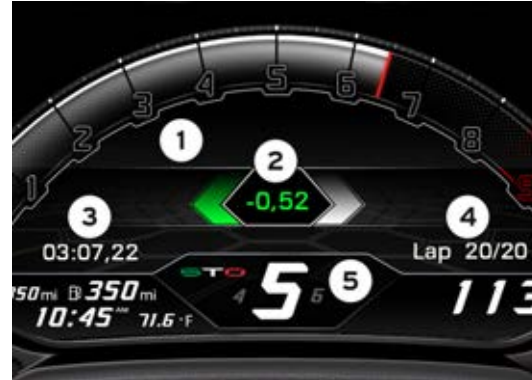
Fig. 43 Instrument cluster: session with display in the Bargraph mode.
