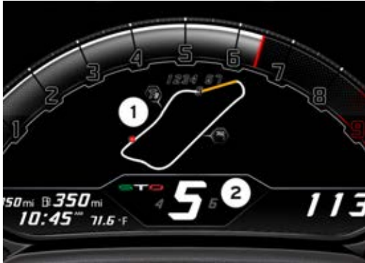
Fig. 40 Instrument cluster: Warm up with display in the Track mode.
