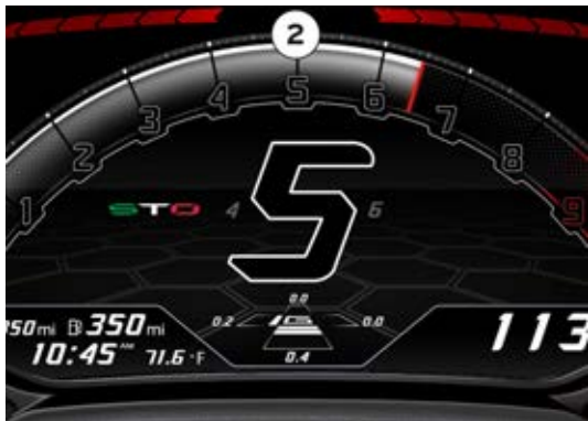
Fig. 9 Instrument cluster: Tachometer LED.
