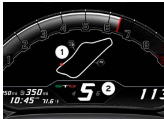
Fig. 39 Instrument cluster: recording a new route with display in the Track mode.
