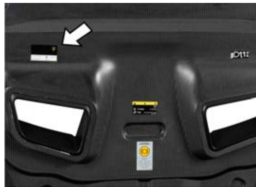
Fig. 151 Paint identification sticker: position and close-up.
