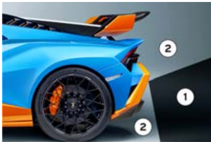
Fig. 98 Rear view camera. Sector covered by camera (1) and sectors not covered (2).
