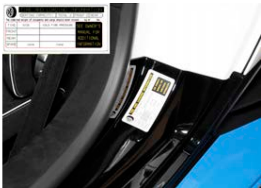
Fig. 166 Location of the tire pressure sticker on the inside of the driver's door.
