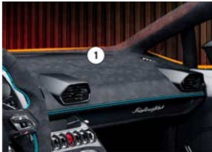
Fig. 126 Position of airbag on passenger's side: on the instrument panel.
