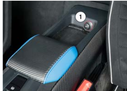
Fig. 82 Storage compartment with cigarette lighter/ electrical socket in the rear part of the center console.
