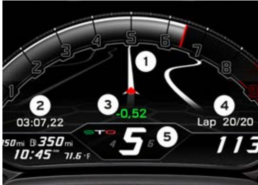
Fig. 42 Instrument cluster: session with display in the Track mode.
