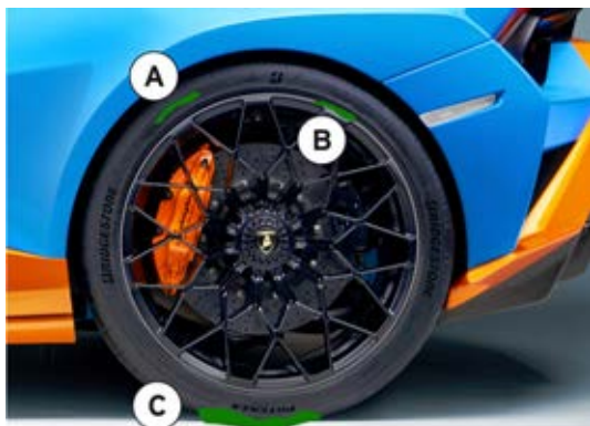
Fig. 181 Damage that cannot be repaired with the Tire Mobility System (TMS).
