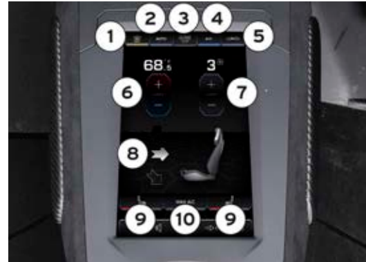
Fig. 92 Air conditioning controls.
