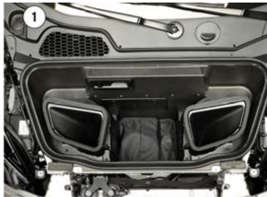
Fig. 165 Luggage compartment: filler pipe for the windshield wiper/washer reservoir.
