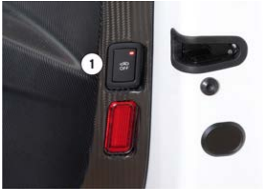
Fig. 57 Switch for disabling the interior monitoring system.
