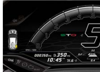
Fig. 28 Instrument cluster: identification of a tire with a large loss of pressure.
