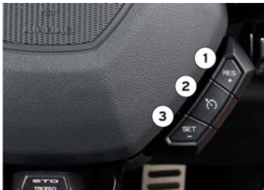
Fig. 45 Cruise Control controls.
