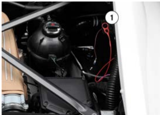
Fig. 155 Opening the fuel door manually in case of emergency.
