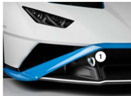
Fig. 190 Front bumper: towing hook installed.
