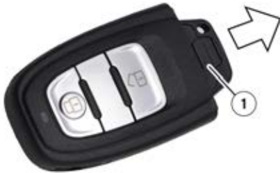
Fig. 55 Separating the electronics in the master key.
