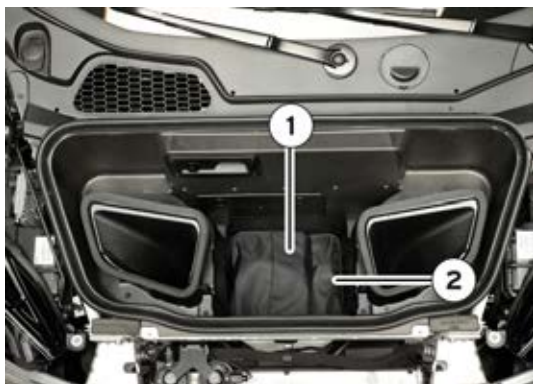
Fig. 179 Location of tool kit in the luggage compartment.
