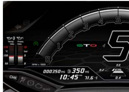
Fig. 110 Instrument cluster: engine off (stop cycle).
