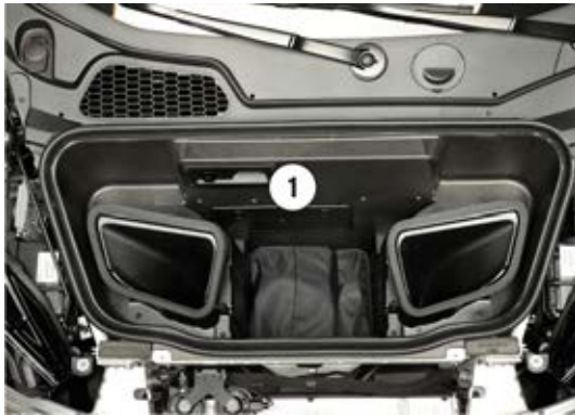
Fig. 164 Luggage compartment: battery terminal access point.
