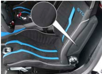
Fig. 130 Marker showing the location of the combined side head/torso airbags in the seats.
