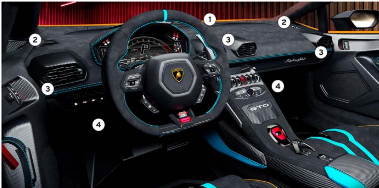
Fig. 91 Instrument panel: air vents.
