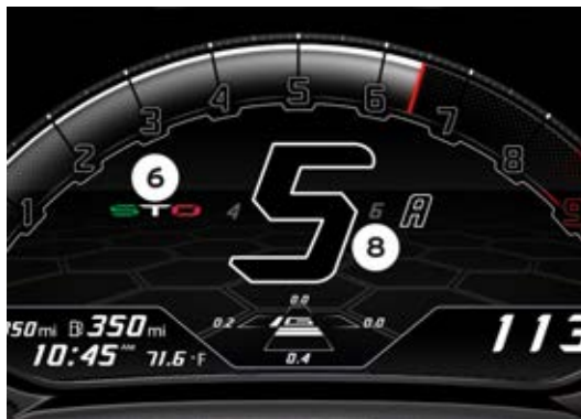
Fig. 109 Display of driving mode (6), gear currently engaged and gear changing mode (8).
