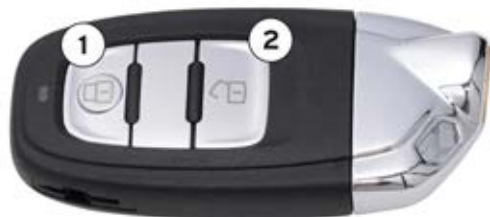
Fig. 52 Key with remote control: functions of the buttons.
