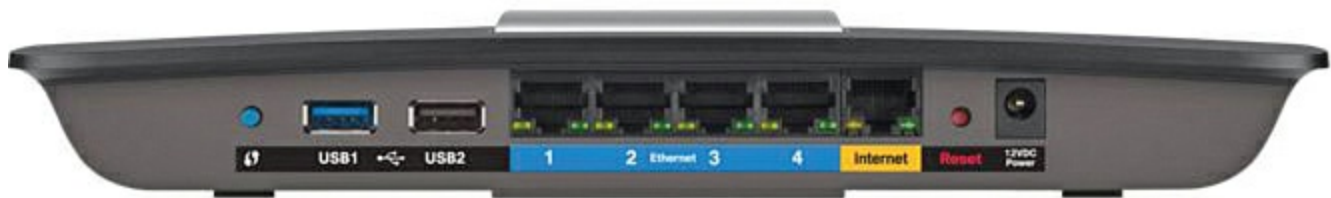
FIGURE 7.1 A wireless broadband router for a small network
