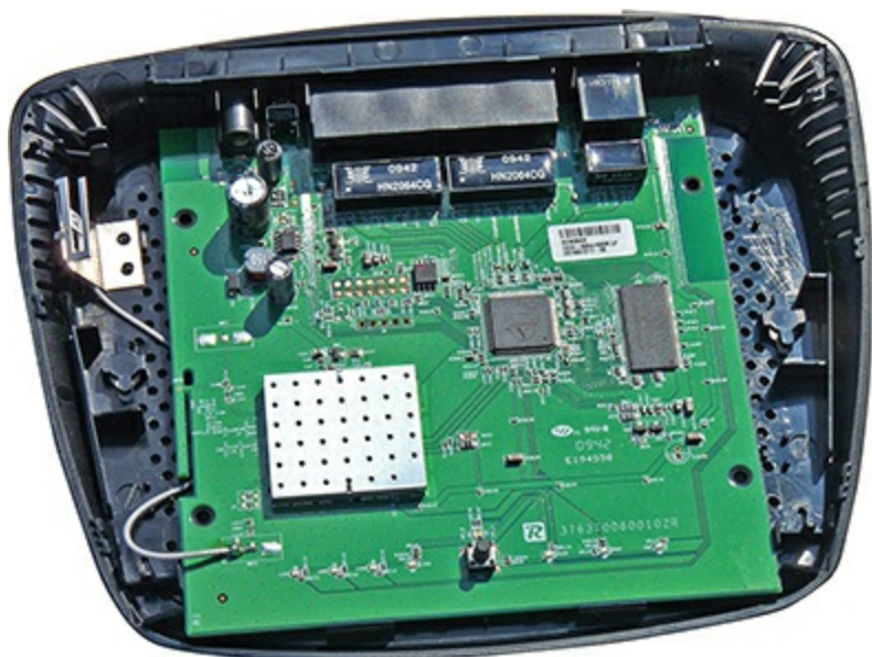
FIGURE 7.2 The antenna is the wire and metal component on the left
