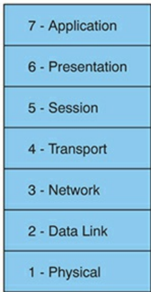
FIGURE 2.1 The OSI seven-layer model
