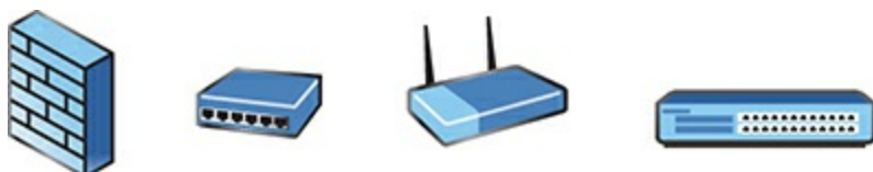
FIGURE 9.1 Diagram symbols for a firewall, a hub, a router, and a switch
