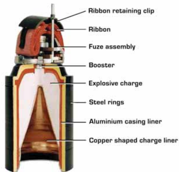
Figure 1: Cross section of an M85 bomblet.
