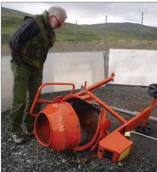
Figure 22: A total of 32 cement mixers were blown to pieces by unarmed and so-called 'non-hazardous' duds during sensitivity tests in Norway, which included both M85 duds and DM1383 duds. 1 in 4 of the unarmed duds exploded during the cement mixer tests. Photo: Grethe Østern/NPA
