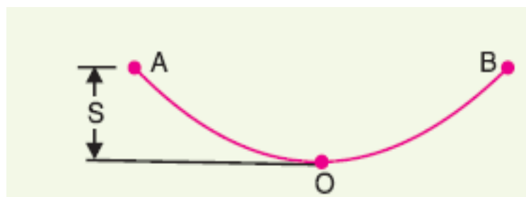
Fig. 2.5 Sag in Overhead lines
