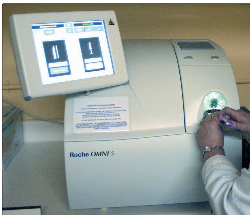
Fig 24.1 Blood gas analyser.
