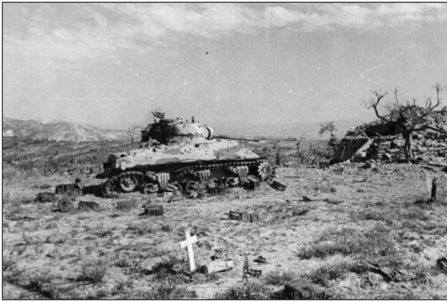
Private Tom Sherlock from the 27th Machine Gun Battalion took this photo of an abandoned Sherman III. As well as a penetration in the side and scorings of bullet marks, it appears to have run off its right track after hits to its suspension.
