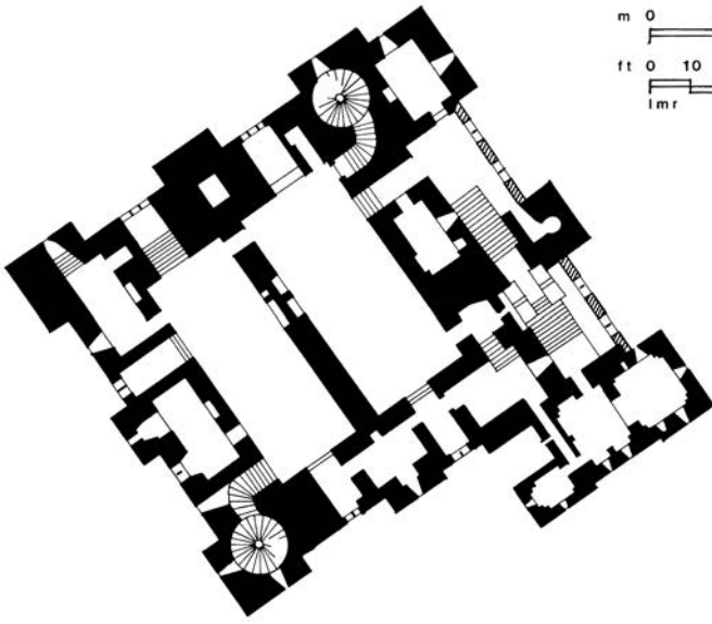
14.5. Keep of Dover Castle, Dover, England, 1180s. Plan. Freestanding keep towers were the basis of later castle construction. Some were square, as in this example, while others were cylindrical. Drawing: L. M. Roth.
