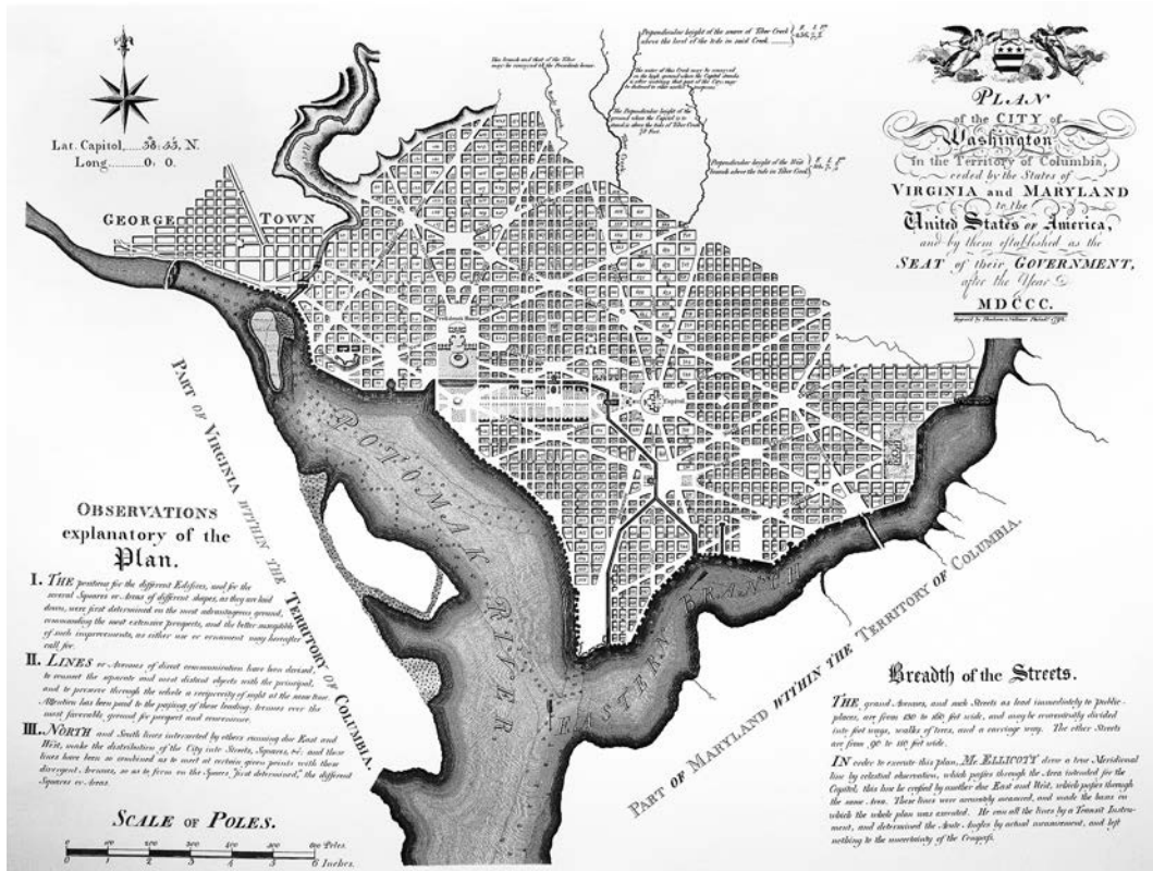
17.20. Charles Pierre L'Enfant, Plan for the City of Washington in the Territory of Columbia, designed in 1791, shown as slightly adjusted by surveyor Andrew Ellicott and published in 1792. Placing the two most important government buildings on low hills, L'Enfant connected them with a diagonal street, generating comparable radiating streets focusing on the two focal points, and then overlaying an orthogonal grid of streets. From Plan for the City of Washington in the Territory of Columbia (Philadelphia, 1792; Historic Urban Plans, Inc., Ithaca, New York, USA).
