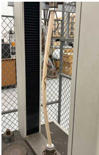
Figure 5. Specimen #6 buckling under compression.
