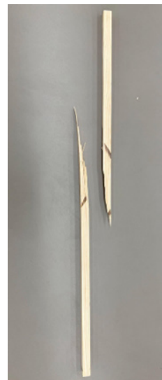
Figure 6. Specimen #3 ruptured after compression.
