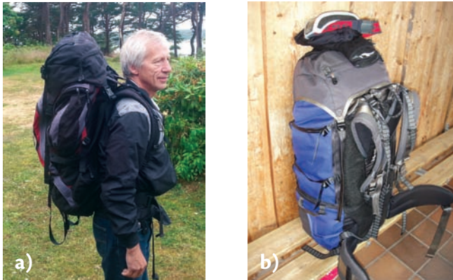
Figure 24.3 a, b) A modern backpack (rucksack) is equipped with a system of straps as it is constructed to unload a large part of the shoulder weight to padded hip belts, leaving the shoulder straps mainly to stabilize the load. There is also a tight stretched netting panel, which prevents contact between the metal frame and user's back.
