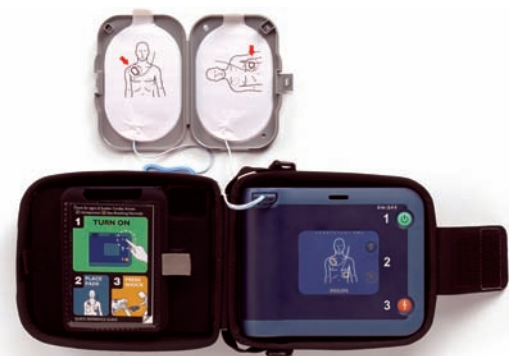
Figure 7.2 a, b) An automated external defibrillator (AED) should be available where sport of many kinds are being played. A heart-starter should be used by whoever comes first on the scene when there is suspicion of a heart problem. A commonly used type is HeartStart FRx, which is used by the Swedish Football Association's National teams. (Courtesy of Philips from Laerdal Medical.)
