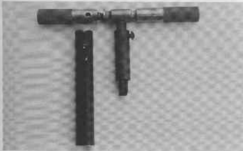
PHOTO 14: Complete reamer assembly. Sleeve is shown in position with reamer guide alongside.
