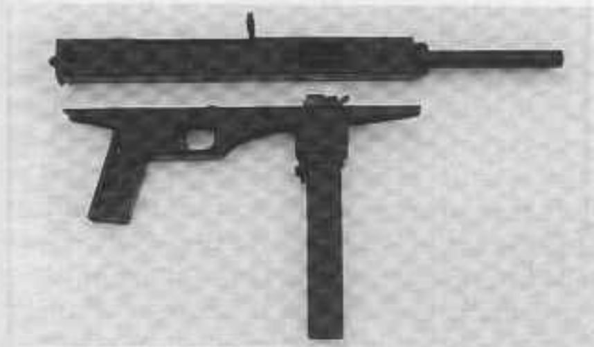
PHOTO 54: The two receivers ready to be bolted together.
