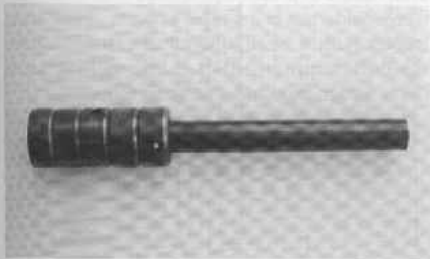
PHOTO 17: Barrel fully assembled with all collars fitted.
