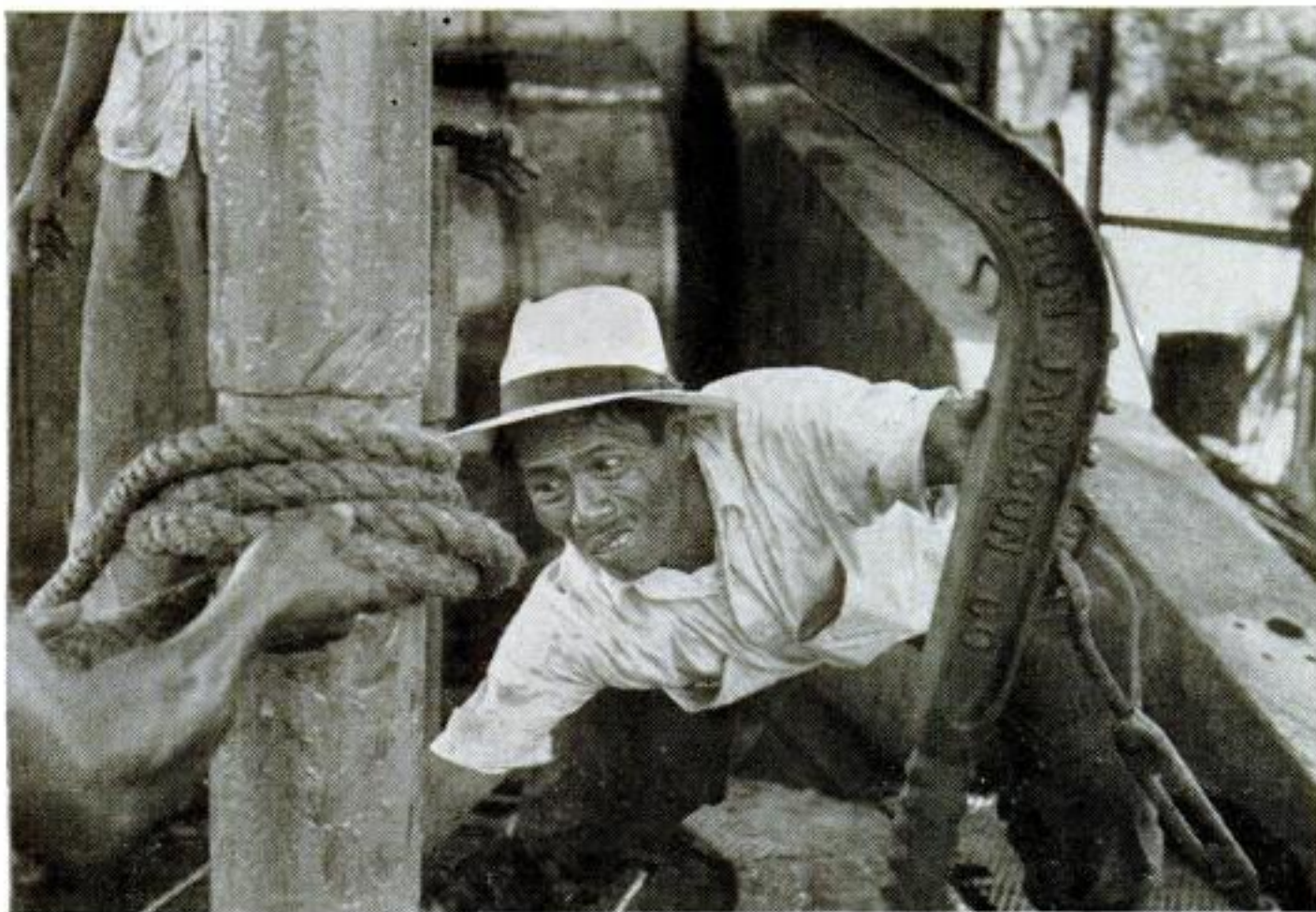
OIL WORKER bends to connect a new pipe to the drilling rig at a Palembang field. This big Standard-Vacuum field was brought into production 28 years ago.
