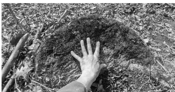
Rough-hewn millstone, which was broken during processing and then discarded. There are a few more locations on the mountain with pieces of broken millstones. Stonemasonry on the mountain has been documented since the end of the 19th century and was limited to the production of millstones for manual grinding. The stone suitable for this is quartz sandstone, which is abundant on the mountain. Given the fact that this type of stone was used to make millstones in the Roman period and
