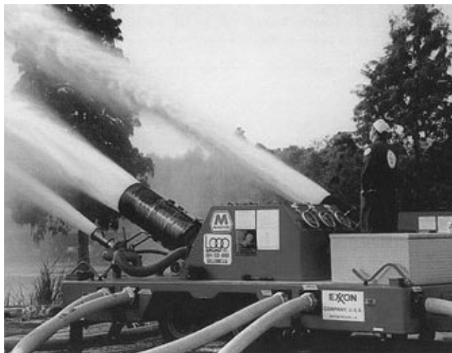
Figure 9—Three Monitors with Large to Very Large Flow Capacity
