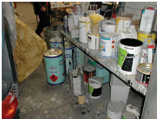
Figure 1.16 Highly flammable substances
