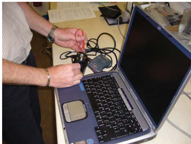
Figure 8.13 Portable appliance testing
