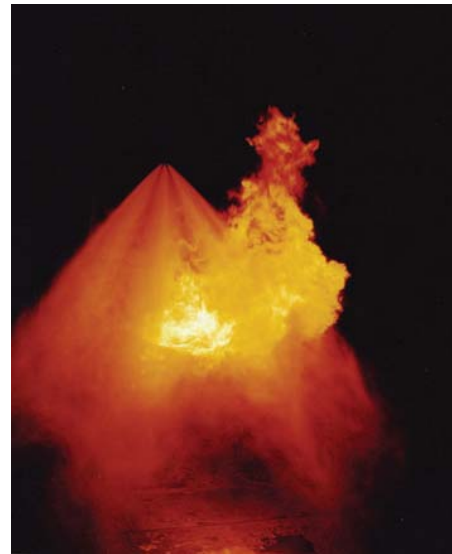
Figure 9.67 High pressure water mist system in operation
