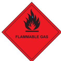
Figure 7.8 Typical flammable gas sign
