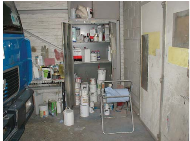
Figure 8.5 Poor storage arrangements for flammable materials
