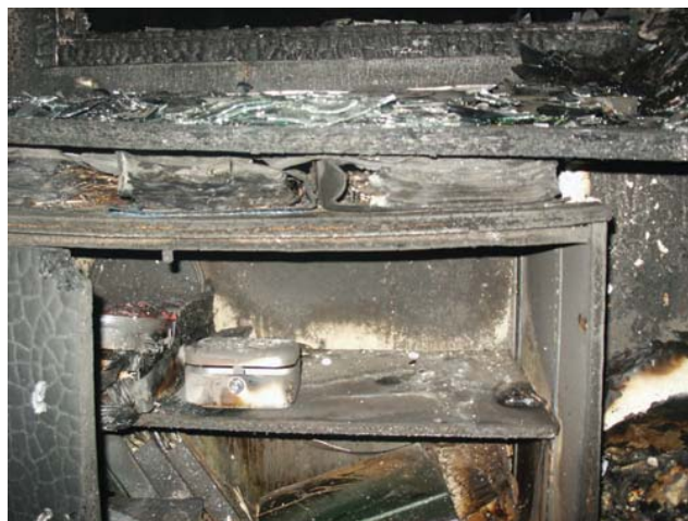
Figure 12.14 Cash box damaged by fire
