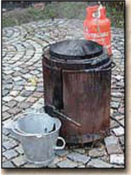
Figure 8.30 Tar boiler used to heat bitumen
