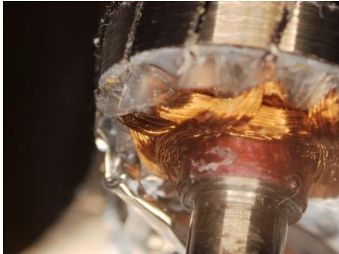
Figure 46: Coil exposed after End Cap removal
