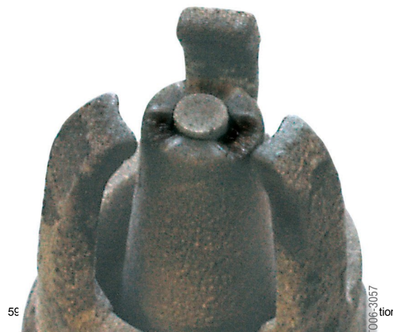
58 - N53 engine spark plug in good condition
