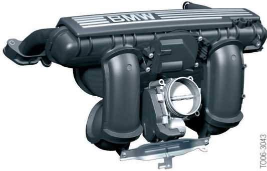
20 - Intake air manifold with throttle valve on engine N53
