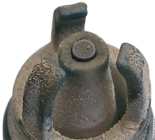
58 - N53 engine spark plug in good condition
