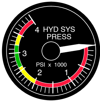
AUXILIARY HYDRAULIC SYSTEM PRESSURE GAGE
