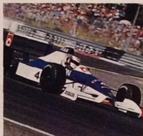
The Williams FW11, top, was the first to feature rear diffusers, while the 1990 Tyrrell 019, above, created quite a stir with its anhedral nose and raised middle chassis section. Below, Nigel Mansell in the Williams FW14 that came so close to the title last season
