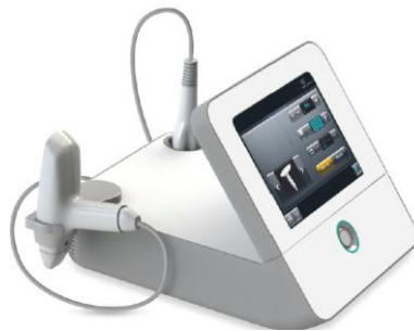
Figure 4-3 Applicators in its cradle
