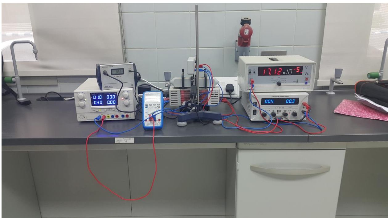
Image (2): The electromagnet, the power supply that provides the sample current and the multimeter that measures the Hall voltage.
