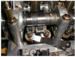
4. Rotate the crank 180 degrees clockwise (the cam pulleys will rotate 90 degrees), the next cylinder in the firing order is **#3**, so the marks will look like on the next picture. Proceed to clearance adjustment just as you did for cylinder 1.
