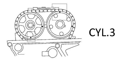
5. Rotate crank 180°, clockwise always, and perform adjustment for cylinder #4:
