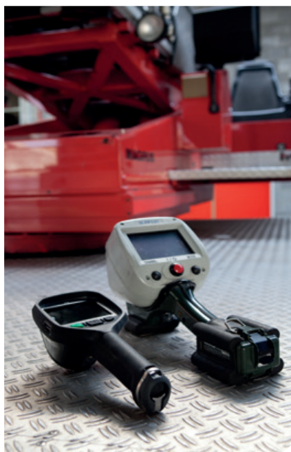
FLIR K50 next to the FireFLIR. Although the FLIR K50 is the preferred tool due to its small size and light weight, the FireFLIR is still proving its worth after 10 years of hard use. It was extensively used during a fire at the Kalmthout Heath in 2011.
