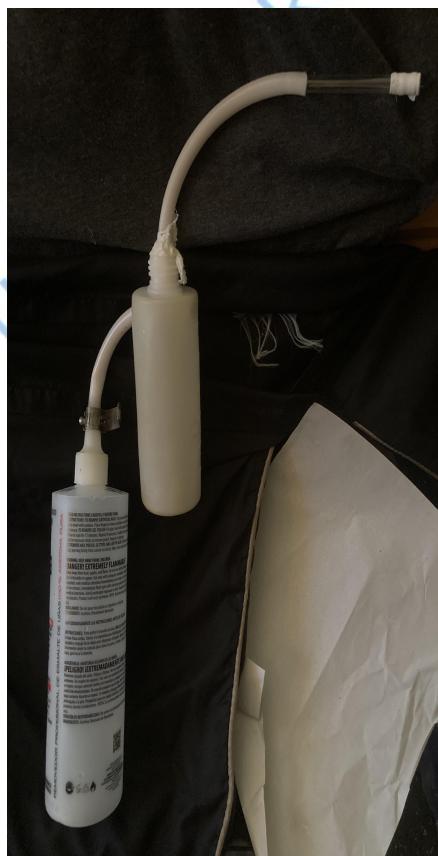
Example photograph of a DIY Hydrogen Chloride generator and in-line drying chamber.
