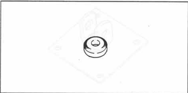
Valve Seat Cutter, 32^\circ - \phi 30 : 57001-1120
