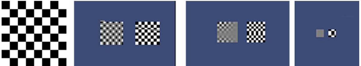
Figure 4-2. The checker map (left). In the three blocks to the right of the checker map, the MIP-mapped texture appears on the left and the non-MIP-mapped texture is on the right, with the quads drawn farther back in space each time
