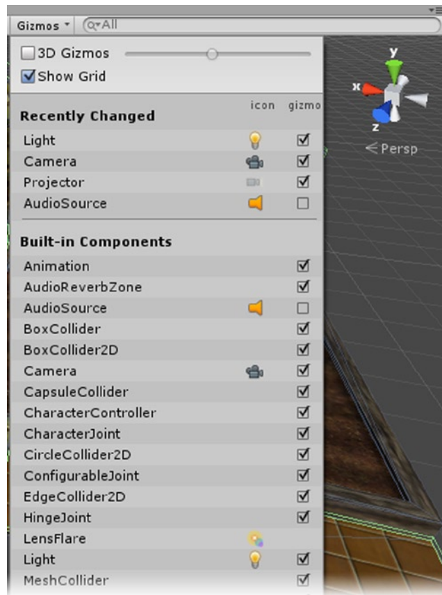
Figure 7-3. The Gizmos drop-down list, where icon visibility and style can be affected
