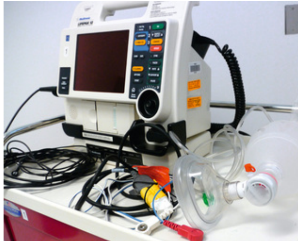
FIGURE 38-21 The LifePak device contains a monitor, a defibrillator, and a transcutaneous pacemaker. Source: Science History Images/Alamy Stock Photo.
