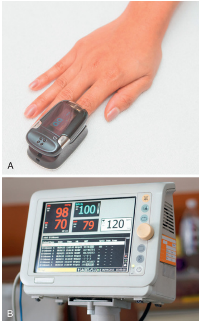
FIGURE 28-7 A , Portable pulse oximeter displays oxygen saturation ( \text{SpO}_2 ) and pulse rate. B , A pulse oximeter displays the oxygen saturation and pulse rate as a digital reading. Sources: A, © Can Stock Photo/praisaeng. B, © Can Stock Photo/masuti.
