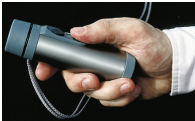
FIGURE 29-12 Artificial larynx. Battery-powered electronic artificial larynx for a patient who has had a total laryngectomy. Source: Courtesy CLG Photographics, Inc. St. Louis.
