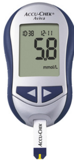
FIGURE 52-9 A blood glucose monitor (Accu-Chek Aviva) is used to measure blood glucose levels. Source: Courtesy Roche Diagnostics Canada, Laval, QC.
