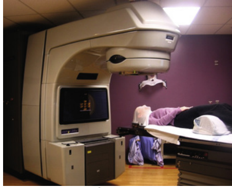
FIGURE 18-14 Linear accelerator. Varian Clinac EX linear accelerator with multiple photon and electron energy levels available for use according to the treatment plan. Patient is positioned on radiation treatment table for treatment of head and neck cancer. Source: Courtesy Jormain Cady, Virginia Mason Medical Center, Seattle, WA.
