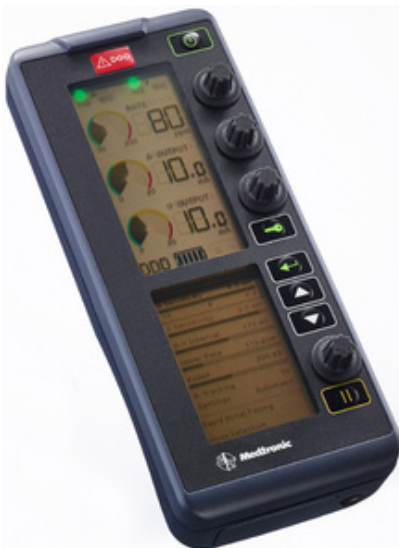
FIGURE 38-25 Temporary external, dual-chamber demand pacemaker. Source: © 2017 Medtronic.
